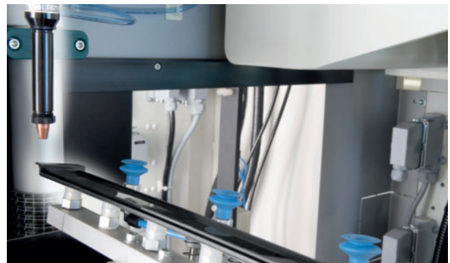
Fig. 3. Separating the sprue by laser (using the example of a transparent display window)
