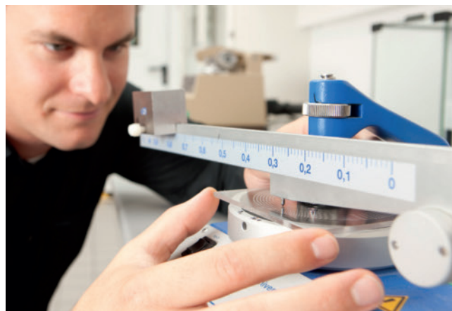
Fig. 5. Testing scratch hardness as per Erichsen 413
